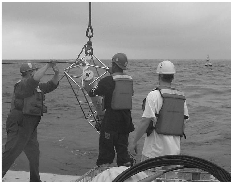
Deployment of instrumentation on Bermuda testbed mooring.
