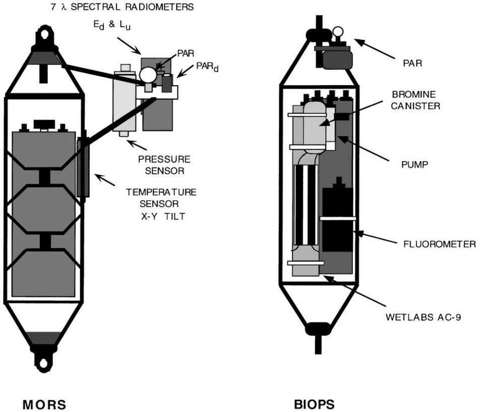
Fig. 2. Bio-optical instrumentation packages: MORS and BIOPS.
