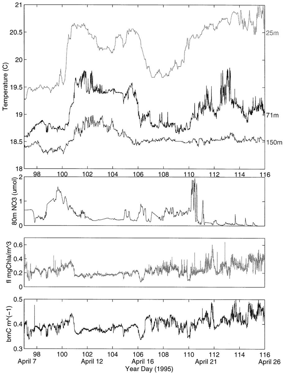
Fig. 7. Time series of (a) temperature at 25, 71, and 150 m, (b) nitrate concentration at 80 m, (c) chlorophyll fluorescence at 71 m, and (d) attenuation coefficient at 660 nm ( $c(660)$ ) at 71 m.
