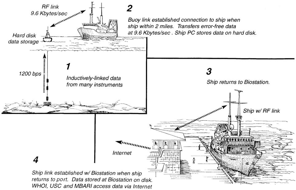
Fig. 5. High-speed RF link from mooring buoy to ship to shore.
