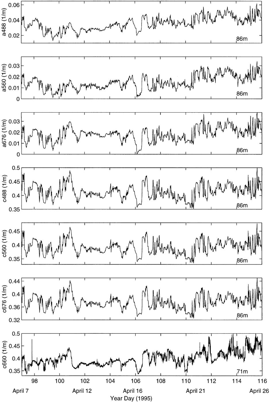
Fig. 10. Time series of absorption and attenuation coefficients at 86 m for selected wavelengths (488, 560, and 676 nm) and  $c(660)$  at 71 m.
