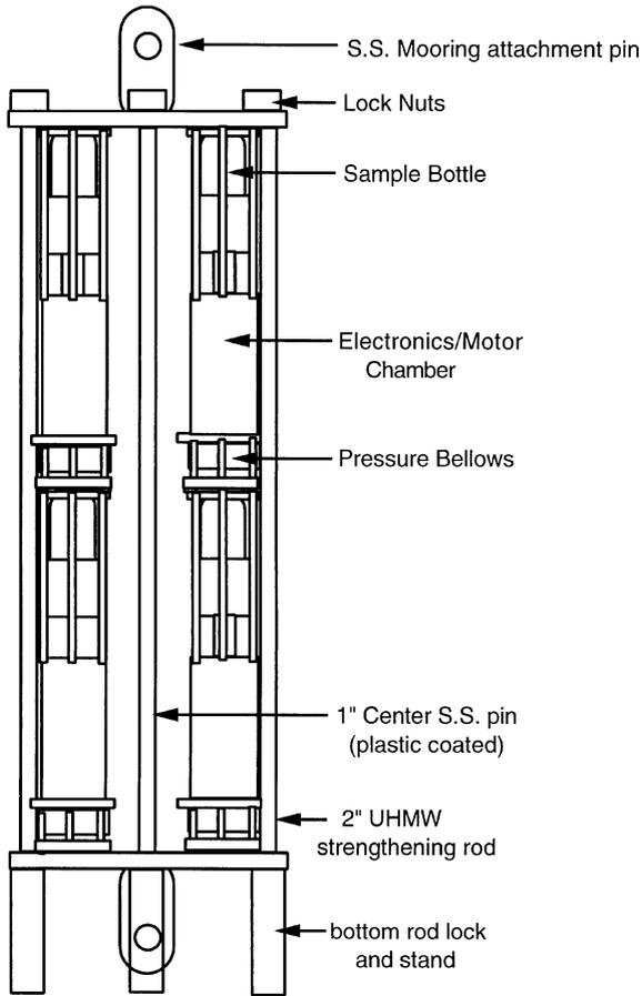
Fig. 4. Moored In situ Trace Element Serial Sampler system (MITESS).
