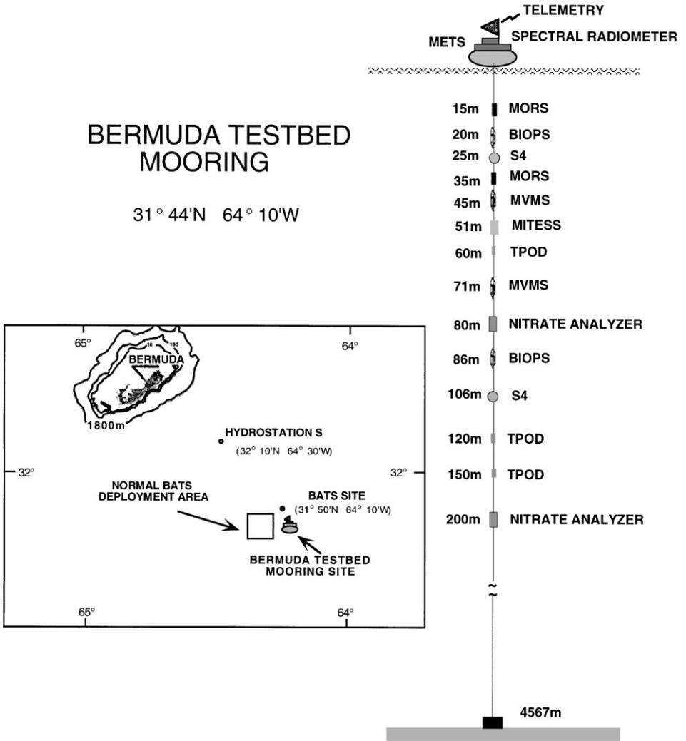
Fig.1. Bermuda Testbed Mooring configuration for the third deployment, 6 April–24 August 1995. Instrumentation systems are described in text. Geographic site of mooring is also shown.
