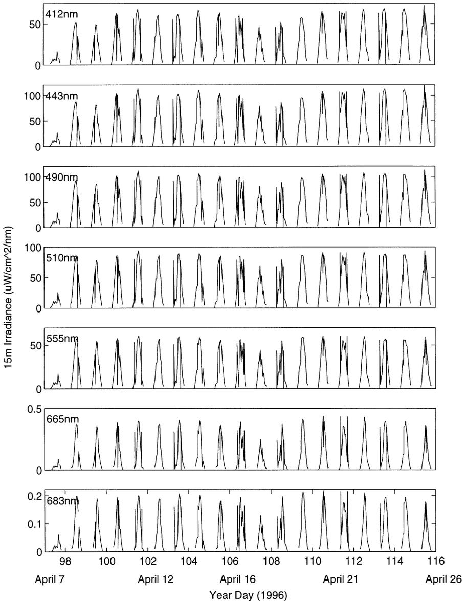
Fig. 9. Time series of downwelling spectral irradiance at 15 m for wavelengths of (a) 412 nm, (b) 443 nm, (c) 490 nm, (d) 510 nm, (e) 555 nm, (f) 665 nm, and (g) 683 nm.
