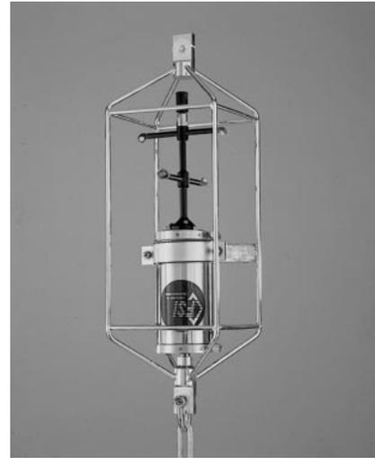
FIG. 2. Photograph of the FSI 3D-ACM.
