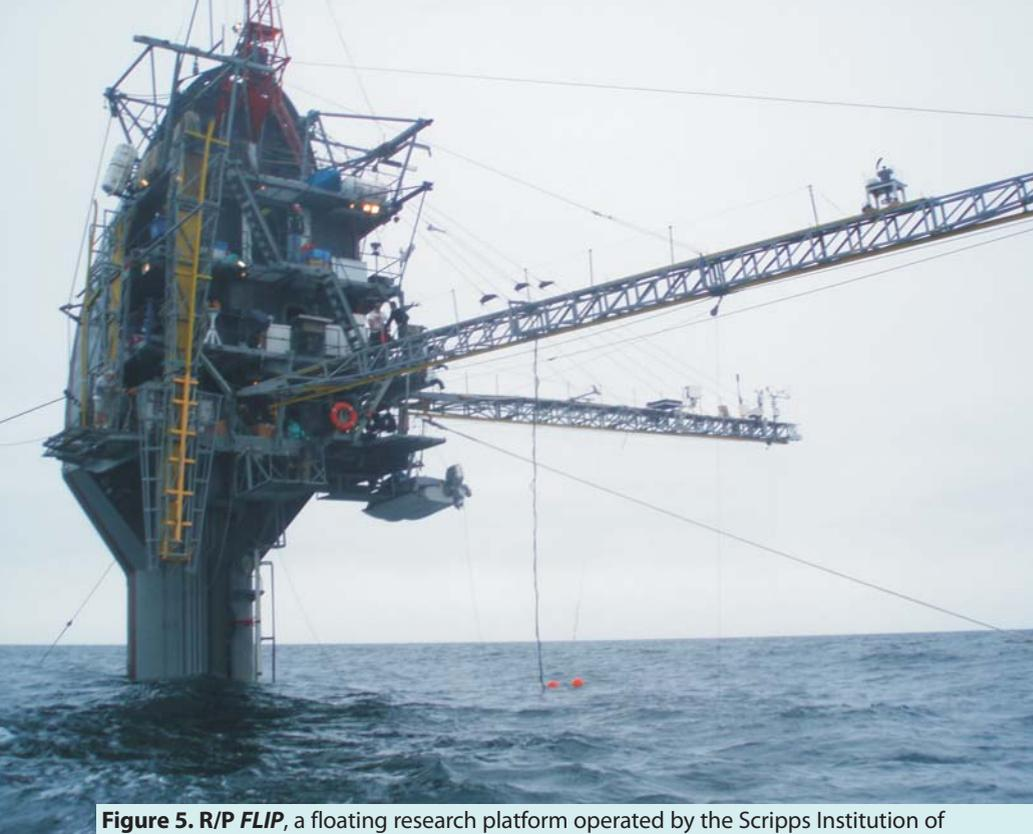
**Figure 5. R/P FLIP**, a floating research platform operated by the Scripps Institution of Oceanography, is an extraordinarily stable platform for the deployment of multiple research instruments at sea. It's a towable sea-going vessel 108 meters long that becomes the tall, stable tower shown in the photo when its aft ballast compartments are flooded to flip the vessel bow up. (Photo by Kyla Buckingham.)
