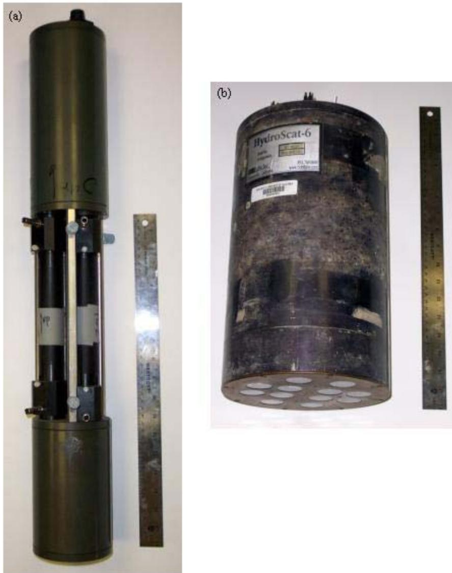
Figure 3. Photographs of instruments that measure inherent optical properties: (a) WET Labs, Inc. nine-wavelength absorption-attenuation meter (ac-9), and (b) HOBI Labs six-wavelength backscattering instrument (HydroScat-6).
