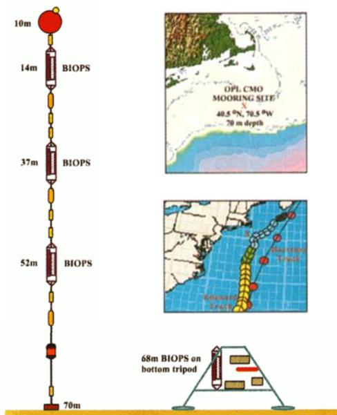
**Figure 1.** Geographic map indicating site of mooring and tripods used for the present study. Map showing tracks of Hurricanes Edouard and Hortense. Mooring and optical tripod schematic diagrams.
