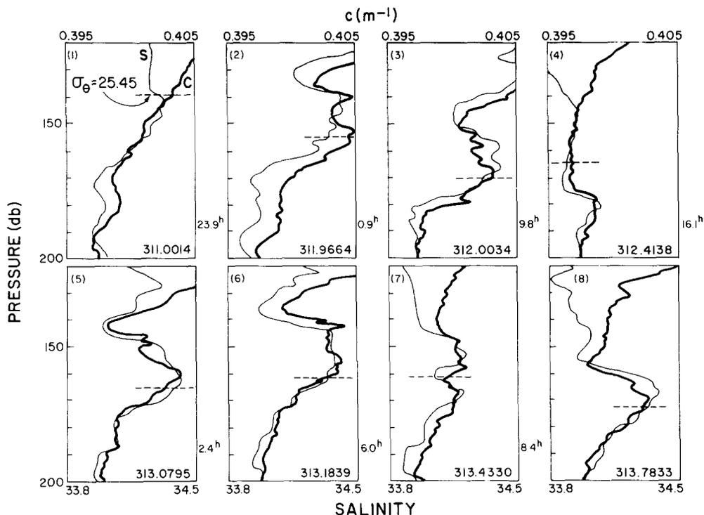
Fig. 3. Sequence of vertical profiles of  $S$  (thin line) and  $c$  (bold line). Time in days is given at lower right of each panel and time interval in hours between profiles is given between panels. Numbers at upper left of each panel correspond to arrows along time axis in Fig. 2A. Depth-pressure range of these profiles is indicated by dashed rectangles at lower right corners of Fig. 2A and B. Position of  $\sigma_{\theta}$  25.45 isopycnal is indicated by dashed line segments.
