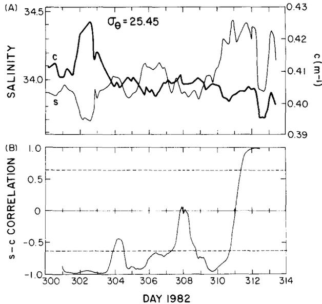
Fig. 4. (A) Time series of  $S$  (thin line) and  $c$  (bold line) on  $\sigma_\theta = 25.45$  isopycnal. (B) Time series of 2 day correlation coefficient between  $S$  and  $c$  on the  $\sigma_\theta = 25.45$  isopycnal. Dashed lines indicate 95% confidence limits for non-zero correlation.
