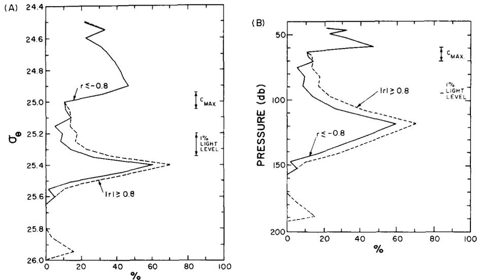
Fig. 7. (A) Fraction of observation time vs  $\sigma_\theta$  for which  $|r| \geq 0.8$  (dashed line) and  $r \leq 0.80$  (solid line) where  $r$  is the correlation coefficient between  $S$  and  $c$ . (B) As in (A) but vs pressure.
