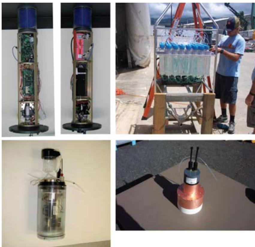
Figure 2. Chemical measurement systems used during the NOPP O-SCOPE and MOSEAN programs. (Upper left) Two views of the MAPCO<sub>2</sub> system that was deployed from the MOSEAN H-A buoy. (Upper right) The Remote Access Samplers (RAS) system deployed from the MOSEAN H-A buoy. (Lower left) The Spectrophotometric Elemental Analysis System (SEAS), which was deployed from the NOAA tsunami mooring. (Lower right) The SubChem phosphate analyzer deployed from the MOSEAN CHARM mooring.
