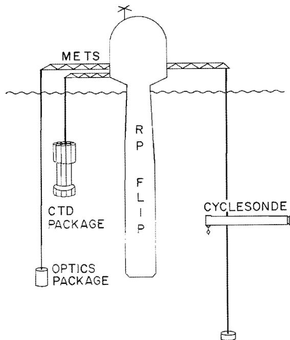
Figure 1. Sampling configuration of the R/P FLIP during the ODEX field study.
