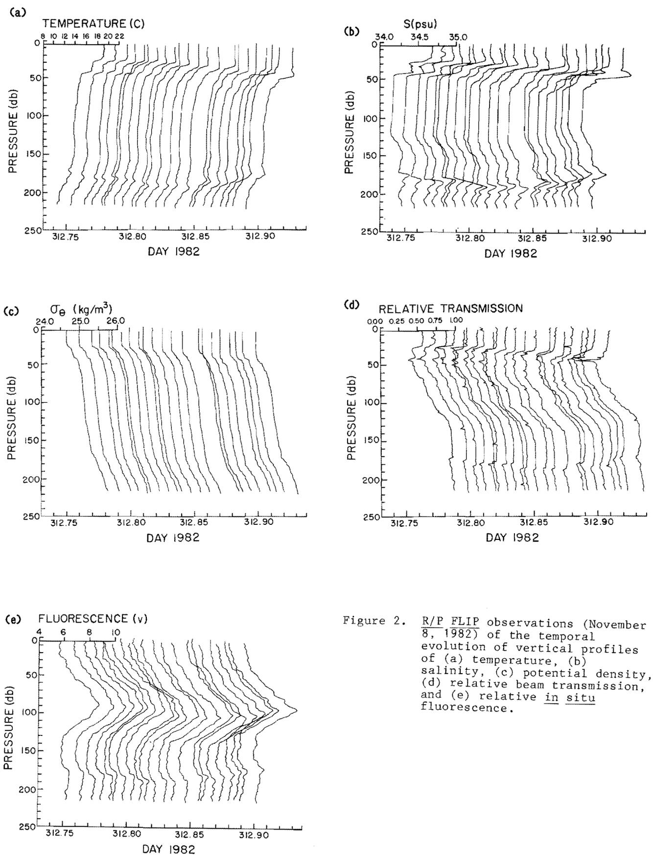
Figure 2. R/P FLIP observations (November 8, 1982) of the temporal evolution of vertical profiles of (a) temperature, (b) salinity, (c) potential density, (d) relative beam transmission, and (e) relative in situ fluorescence.
